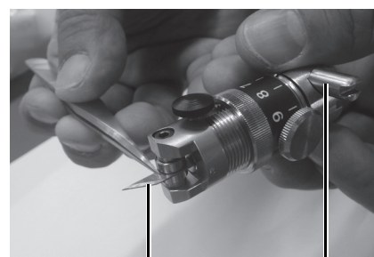
Orientation of blade Stopper screw
