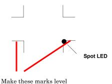
8 When the next sheet is loaded, the plotter detects the register marks automatically and cuts the sheet.
