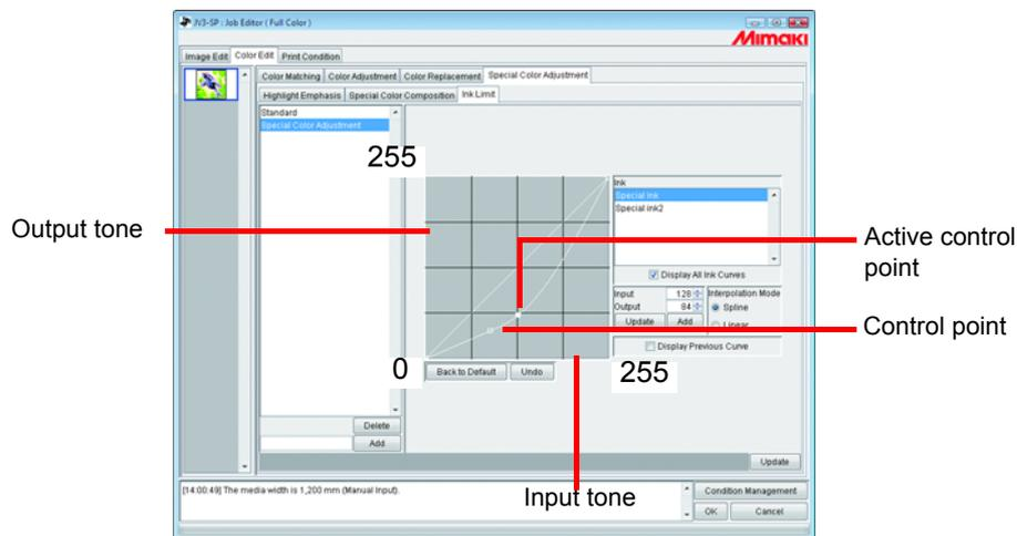
An example of ink curve application when using special colors on the “Gradation” menu in the “Color Replacement” menu.
