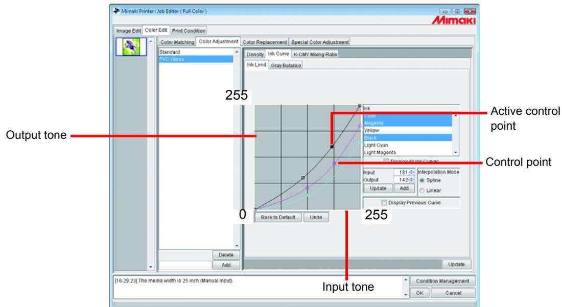
When changing several ink curves at a time, drag a point where the ink curves of several colors are intersecting or adjoining each other. Or push Arrow key to move that control point.
