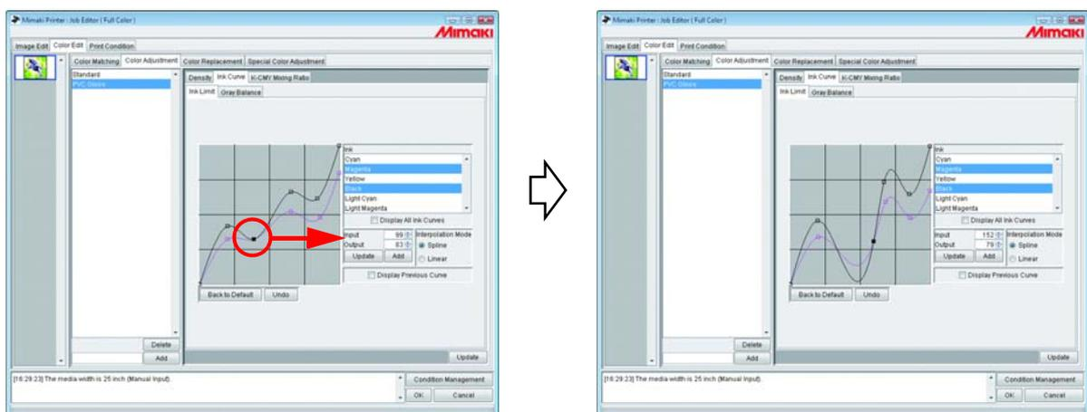
To delete a control point, drag the point to outside the adjacent one. Or push **Delete** key or **Back Space** key.
