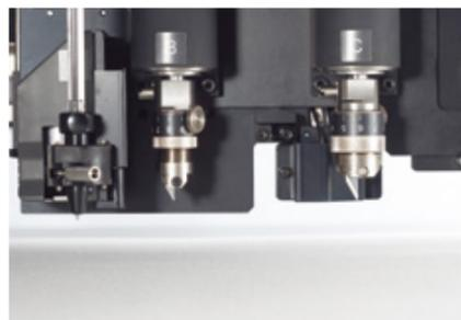
The tangential cutter steers the blades as it cuts. With two types of tangential cutters and fine cut pressure settings a wider range of materials can be cut successfully. Various cutting tools are provided for a range of materials. Any suitable blade available on the market, can be mounted.
